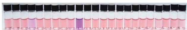
Fig. 2 Color changes of sensor 1·2Zn in 50 mM aqueous HEPES buffer solution (pH 7.4), [ 1·2Zn ] = 35 μM, [PPI] = 35 μM, [other anions] = 175 μM. Anions from left to right: none, AMP, ADP, ATP, PO 4 3- , HPO 4 2- (Pi), H 2 PO 4 - , PhPi, NPhPi, PPI, F - , Cl - , Br - , I - , NO 3 - , SO 4 2- , HCO 3 - , CH 3 CO 2 - , citrate, N 3 - , ClO 4 - , S 2 O 7 2- , C 2 O 4 2- .
